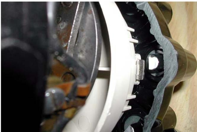
I pulled out my stash of spare distributors and started my test with a '62 340 horse (1110985) unit. I installed the white Delco rotor button and my new Borg Warner cap. As best I could determine, the spark gap was approximately .105".
