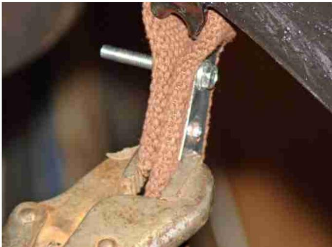
**strap/plates going the wrong direction.** Once you remove the bolt, in order to get the rivet in place you may have to use an electric drill to clean the hole out. If so, select a drill bit the same diameter as the rivet and be careful not to enlarge the holes in the rivet plates. Also, when you put the vice grips in place you need to make certain that you leave enough room so that the riveting tool can be placed on the rivet head with no interference.
