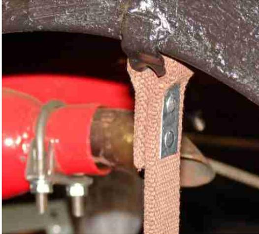
The finished job! The riveting tool does a nice professional looking job of curling the rivet shaft down to the rivet plate. Hopefully, this installation will last another 30 years
