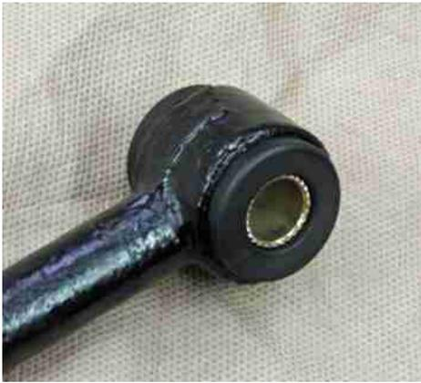
Now, no amount of pressure will make these new bushings as small as the originals. So, reinstalling them can be a bit of a chore. The end that mounts to the frame is no problem as that is merely a bolt and you can slip the bushed strut rod over the bolt and tighten the nut down.
