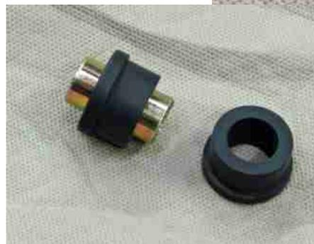
Now, I found that it helped to spray some Silicone lubricant in the holes at the ends of the strut rods – it makes it easier to slip the rubber bushing into the hole. I inserted one half of the bushing, then clamped the assembly in the vise to press the metal insert back into place in the rubber bushing. Hey, I don't have a press – so you use what ya got! Anyway, the vise process worked as you can see.
