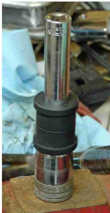
That allows you to separate the rubber bushing for installation. Here I'm driving the metal center section out using a socket to support the bushing assembly and a socket to push the metal center out. You have to put this back together so don't drive the center piece all the way out – once it has moved  $\frac{1}{4}$  to  $\frac{1}{3}$  of an inch you should be able to separate the two parts of the bushing.
