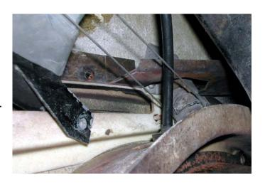
Once you have the four side post bolts and the 8 front frame nuts off you can grasp the frame by the side posts and lift and rock the frame loose from the car. Now a couple of points –
