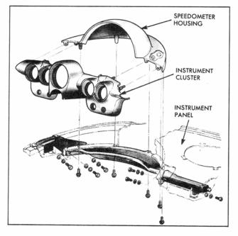
Fig. 10-Exploded View of Instrument Panel
