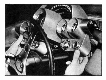
Fig. 11—Removing Instrument Panel from Dash Panel
