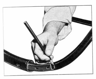
Fig. 5-Marking Position of Upper Frame
