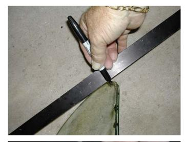
After that it was merely a matter of measuring from the marked spots to the center of the bottom of the windshield. For installation of the rubber channel I don't believe it is necessary to mark the center of the top of the windshield. However, a top center mark will be helpful when remounting the upper frame assembly.
