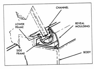
Fig. 8—View of Side Frame-to-Upper Frame Joint
