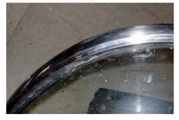
I could press straight down on the bottom frame assembly to seat it on the rubber channel.
