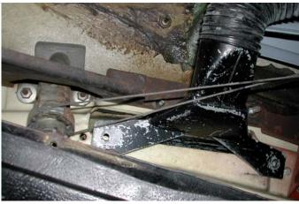
This picture shows the drivers side and even David Copperfield would not be able to get the frame nut off without dropping the defroster outlet – well, perhaps you could if the framework that holds the brake/clutch pedal and steering column were out of the car. It is a very difficult job just to get the defroster nuts off by themselves, getting them back on will be a genuine treat!!!
