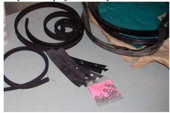
need replacement. The final gaskets to have on hand are spacer gaskets that go under the side posts – these gaskets help adjust the frame to be level on the car. I suspect that not having the correct amount of spacers here results in the broken ears on the bottom of the side post assemblies. Finally, it would be a good idea to have some extra nuts and washers on hand for the reinstallation process – you are gonna drop some of them before this is all back together again!
