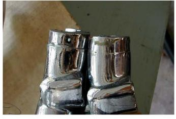
difference in this picture – the left assembly has the visor hole. I drilled and tapped an appropriate hole before I sent the side posts off to be rechromed.
