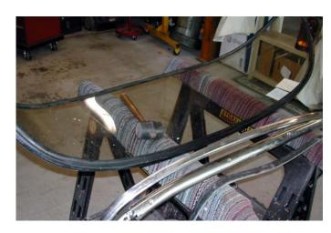
The next move is to clean all the old sealant and putty out of the channels of both the frame and side post assemblies. The sealants used by the General will clean off pretty easily – even after 40 + years the putty was still soft and pliable. If you have a frame where silicone sealer was used it will take a little longer. On the side post assemblies for my '61, there was an ink stamping of a May 19, 1961 date and there was an extra small
