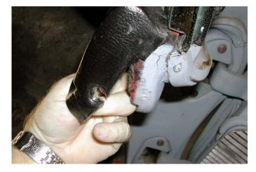
Somewhere in a previous life, someone had the windshield off this car because they had enlarged the access hole so that it is easier to get to the nuts. You can see where the hole was cut with – probably, a key hole saw. Not very professional, but access to the nuts must really be difficult without that hole being enlarged. Once the four ½" nuts are removed from the side frame assemblies, the hard part starts.
