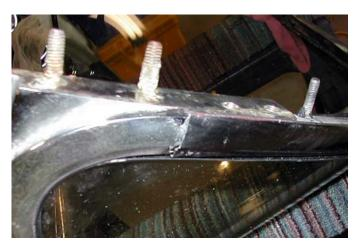
into position so that they will accept the screws. Be very careful, while there is a rubber channel gasket between the floating anchor and the glass of the window it is possible to get heavy handed and push a sharp scribe through the rubber and scratch the edge of the glass – if this happens – most certainly the glass will crack! (Been there, done that!!!)
