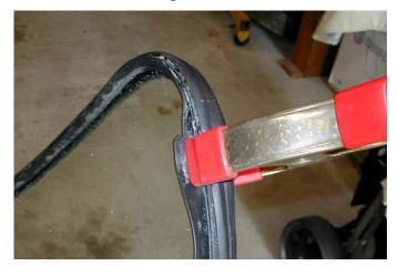
hold the rubber in place on the window while I was fitting the glass to the rest of the channel.
