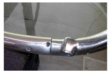
Once the for screws are out, grasp the top of the side post assembly and try to pull it apart from the top frame assembly. If it moves, just pull it out ½" or so. Then grasp the bottom of the side post assembly and try to pull it out of the bottom frame assembly. As above, if it
