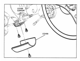
Fig. 9—Mast Jacket Cover and Support
