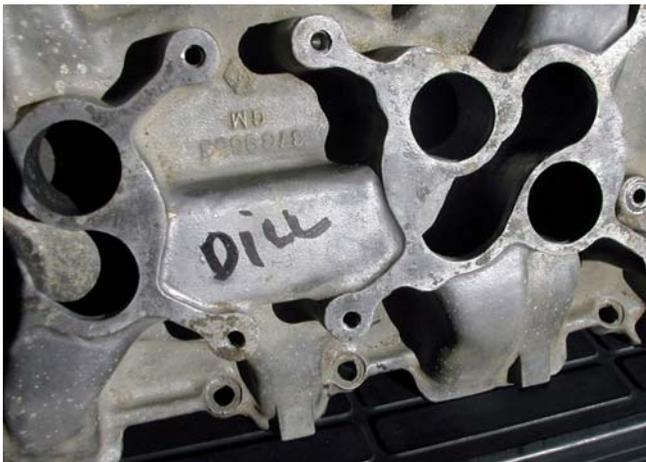
The '57 – '61 manifold (3739653) was changed at the factory to give better efficiency. You can see that the aluminum has been removed between the holes. And, as you can see in this picture, the part number and GM, as well as the snowflake mark are between the two carb bases. This and the firing order found near the oil filler tube are the only obvious markings on the top of the manifolds.
