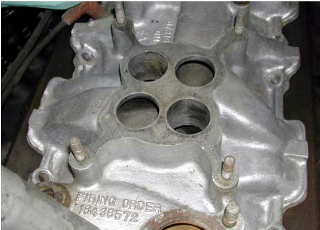
Aside from the part numbers, there was one major difference between the two most common manifolds. The '56 manifold (3731394) had four distinct holes for each carb.
