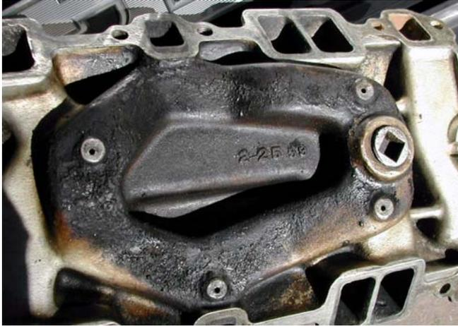
The manifolds are date marked on the bottom side. The marking is under the oil shield which is pinned to the bottom of the manifold. The shield has been removed from this manifold so that you can see the date mark of 2-25-59.
